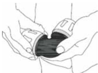
Fully tighten the fitting ring nut without excessively forcing
