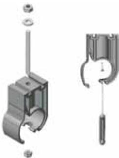
All pipe brackets packagings contain an M8 hexagonal nut to be inserted in the foreseen site inside the bracket (by using a threaded bar). It's also possible to use self-tapping screws with a screw-anchor in case of installation on a wall or concrete
