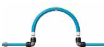
This is the correct application of the installation of expansion joint. It should be facing up and with two elbows aligned. You need also to insert two clips on the pipe aluminum fasteners close to the installation of an expansion joint
