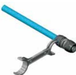
Fully tighten the ring nut and then rotate up to 180° maximum using a pin wrench of suitable size
