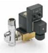
Tierre Group timed condensation drain is normally connected to the pneumatic network at the lowest point and has to be electrically powered. Two grips put on it allow the setting of the gap and the opening time.
